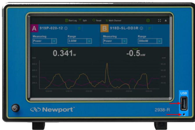
Figure 4-18 Right side of x938 Meter with pinhole highlighted
