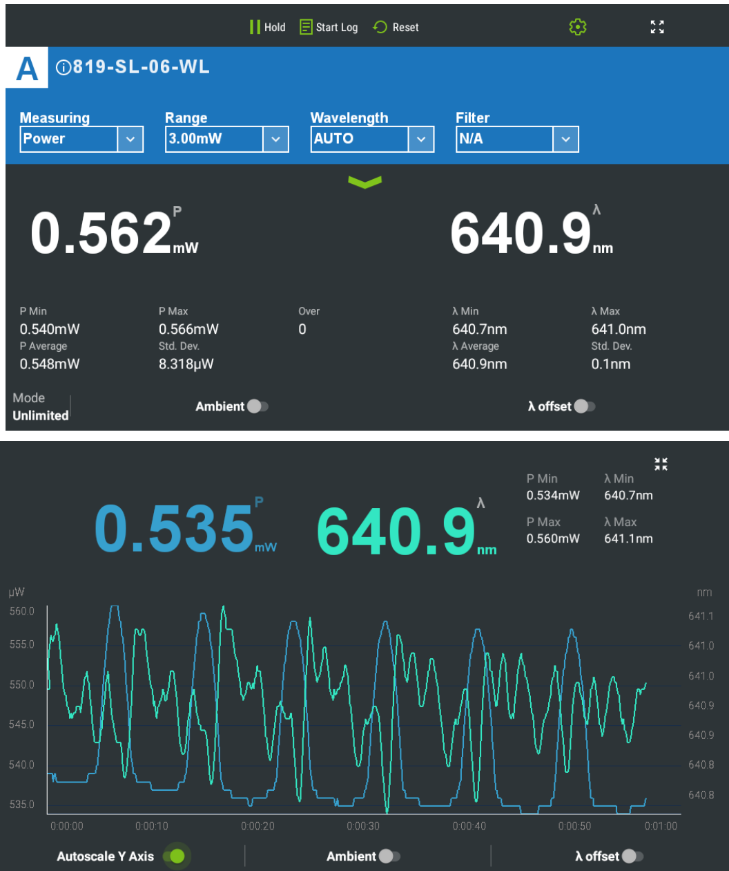
Figure 8-3 819-Examples of display screens for ‘Statistics’ and ‘Expanded Line Graph’ using an 819-WL sensor
